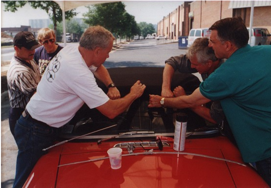
7. Pull top forward and mark center with chalk.
