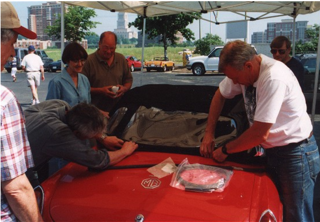
6. Clip rear of new top (with the ever useful, zip-out backlight).
