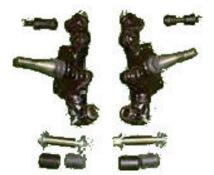
allows the wheel to pivot when the steering wheel is turned. It has a ring at the top which anchors to the shock absorber arm and a hole at the bottom for the fulcrum pivot to secure this end. This is a pretty durable system on MGs, provided some sort of grease lubrication was done on the car over the years and usually does not wear excessively (no rubber components). There are grease
