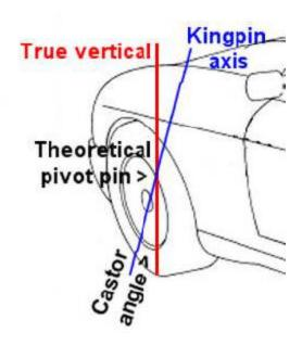
greater the castor angle, the more resistance to turning there is in the steering system and a greater tendency of the car to return to the straight ahead position.
