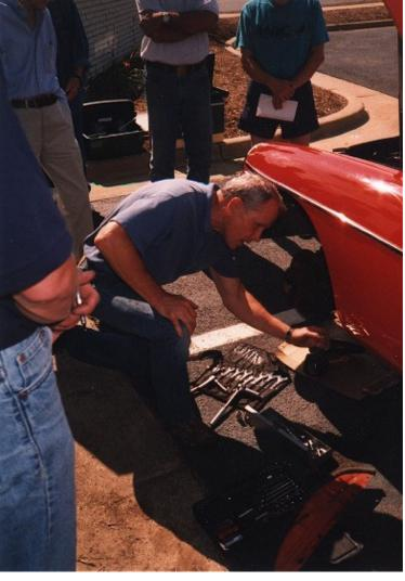
The base of the front wings are cleaned well prior to spraying.
